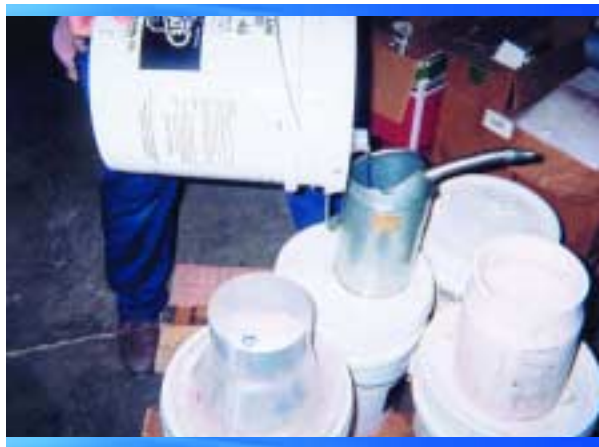
Open top can used for filling oil sumps can be a source of contamination.
