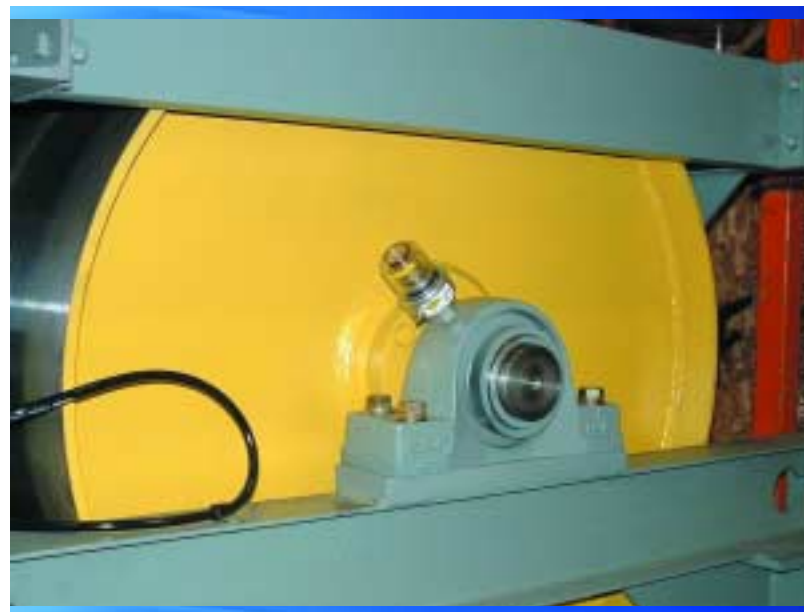
Grease lubricator installed on gear box of a dynamometer.
