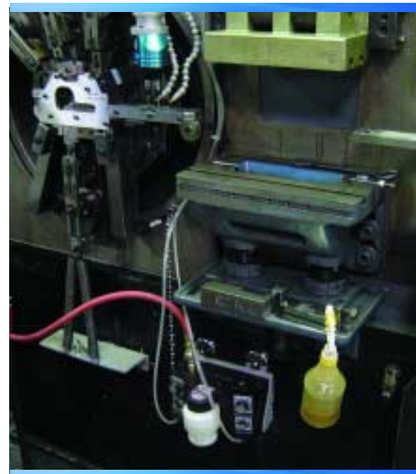
Minimum quantity lubrication used in a tapping workcenter.
