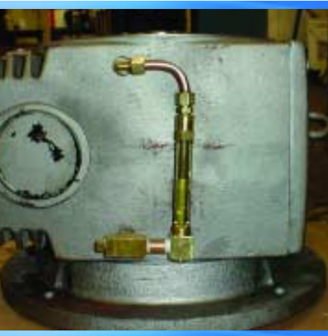
Closed system liquid level gauge with pressure balancing line connected to a gear box housing.
